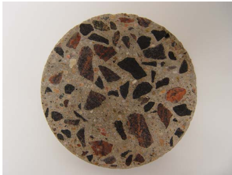
Photo of gasifier residue in concrete
