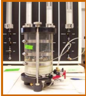
Figure 3. Biogenic Methane Reactor in the Laboratory
